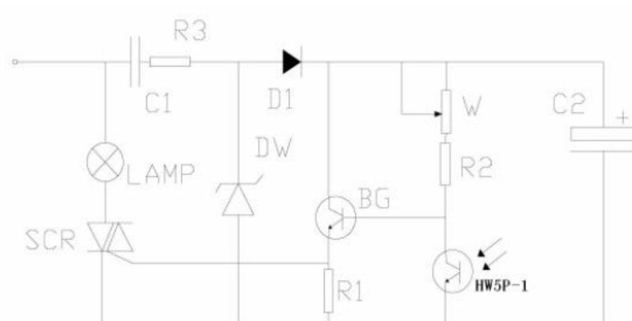
In the chart, capacitor C1, C2, R3 and diode D1 and stable volt DW, composes the simple electric capacity voltage dropping resistor leveling circuit, after meets the circular telegram to obtain about 12V the DC voltage. Triode BG, photosensitive tube HW5P-1 and bidirectional silicon-controlled rectifier and so on, composition photoelectricity switching circuit.
