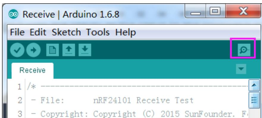
Now, you should see the information received by the nFR24I01 module (on the servo control board) displayed on **Serial Monitor**.
