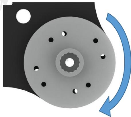
4. Align all holes of the rocker arm and the plate.
