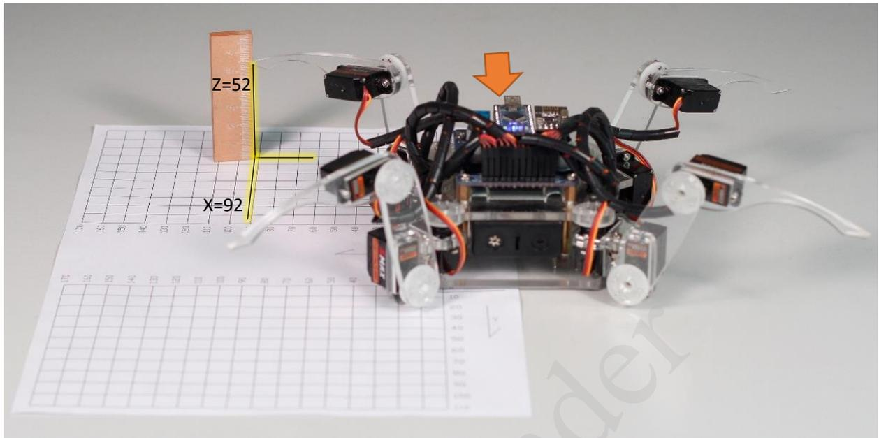
d. Measure the coordinate  $(x, y, z)$  of leg 4. Here it is  $(90, 75, 55)$ .
