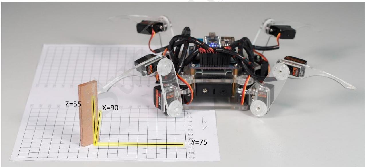
So, the coordinates filled in the array are (108,68,44), (100,65,55), (92,72,52), and (90,75,55), as shown below:
