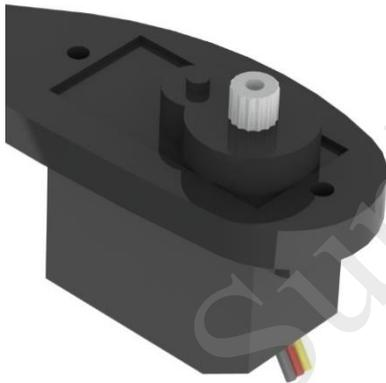
3. Connect these two components with an **M2\*8 screw** and an **M2 nut**.
