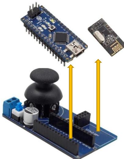
3. Connect the following components with two M3\*14 countersunk screws and two M3 nuts.
