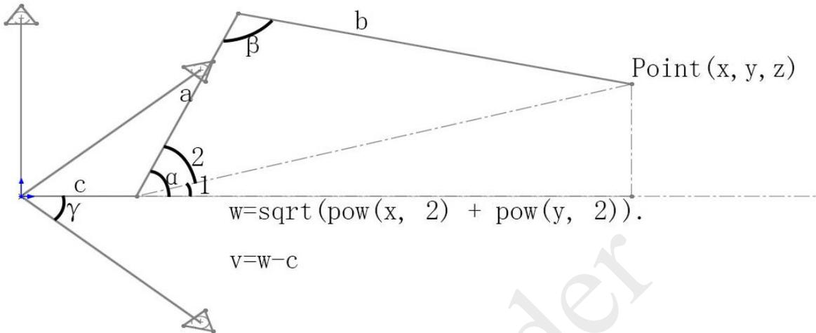
Here we'll only analyze the first quadrant of the leg end: given the end position Point (x,y,z) and segment a, b, c (the length of each segment of the leg), to calculate the rotational angle of the servo  $\alpha$ ,  $\beta$ ,  $\gamma$ . Within,  $\pi/2 \leq \alpha \leq \pi/2$ ,  $0 \leq \beta \leq \pi$ ,  $-\pi/2 \leq \gamma \leq \pi/2$ . In this way, transform these into a basic mathematic model. The proof of the model:
