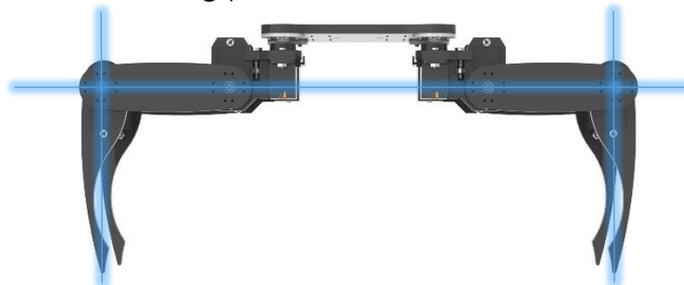
Switch off the SunFounder Servo Control Board. Remove the batteries first, then the battery holder, and finally all the servo wires. Now the joints of the robot can be rotated freely.
