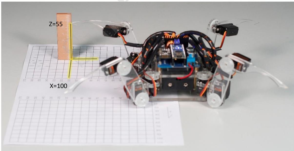
c. Rotate the robot as shown in the following figure, and measure the coordinates  $(x, y, z)$  of leg 3. Here it is  $(92, 72, 52)$ .
