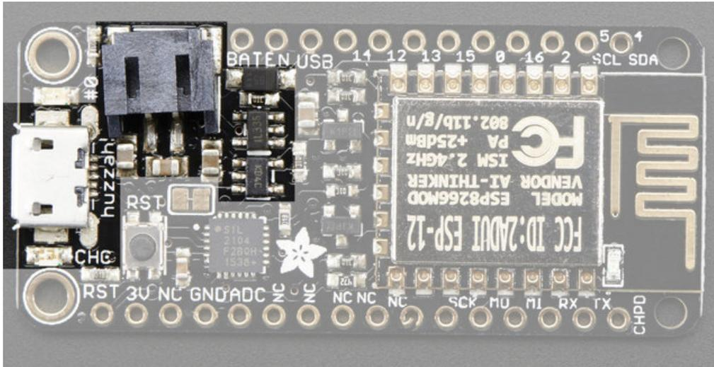
The above shows the Micro USB jack (left), Lipoly JST jack (top left), as well as the 3.3V regulator and changeover diode (just to the right of the JST jack) and the Lipoly charging circuitry (right below the regulator).
