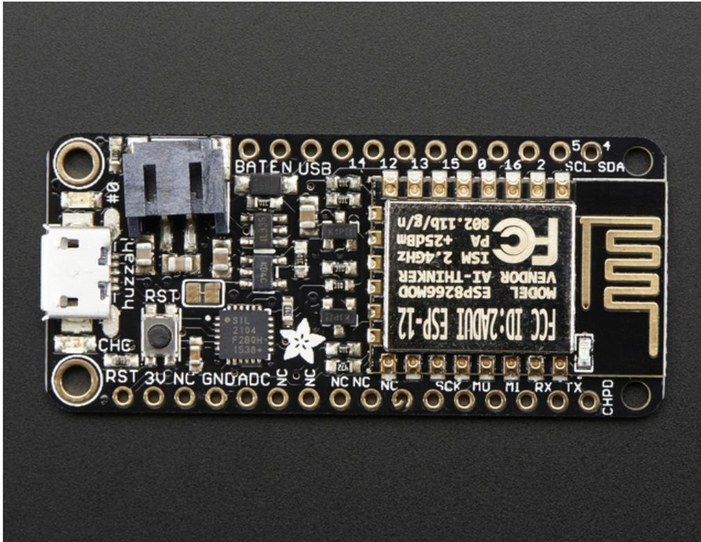
At the Feather HUZAZH's heart is an ESP8266 WiFi microcontroller clocked at 80 MHz and at 3.3V logic. This microcontroller contains a Tensilica chip core as well as a full WiFi stack. You can program the microcontroller using the Arduino IDE for an easy-to-run Internet of Things core. We wired up a USB-Serial chip that can upload code at a blistering 921600 baud for fast development time. It also has auto-reset so no noodling with pins and reset button pressings.
